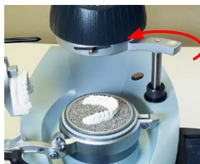
7. ... until it clicks into place (!). The heating switches on.
