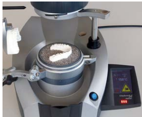
8. Attention , the automated thermoforming process starts. Risk of crushing!
